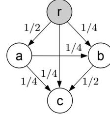
Fig. 2: The edge-capacitated graph  $\widehat{\mathcal{G}}^\pi$  for the wireless network with unit link capacities in Fig. 1 and under the time-average vector  $\beta^\pi = (1/2, 1/4, 1/4)$ . The link weights are the capacities  $c_e \beta_e^\pi$ . The minimum proper cut in this graph has value  $1/2$  (when  $U = \{r, a, c\}$  or  $\{r, b, c\}$ ). An upper bound on the broadcast capacity is obtained by maximizing this value over all vectors  $\beta^\pi \in \text{conv}(\mathcal{S})$ .
