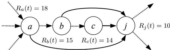
Fig. 4: Under a policy  $\pi \in \Pi^*$ , the set of packets available for transmission to node  $j$  in slot  $t$  is  $\{11, 12, 13, 14\}$ , which are available at all in-neighbors of node  $j$ . The in-neighbor of  $j$  inducing the smallest packet deficit is  $i_t^* = c$ , and  $X_j(t) = \min\{Q_{aj}(t), Q_{bj}(t), Q_{cj}(t)\} = 4$ .
